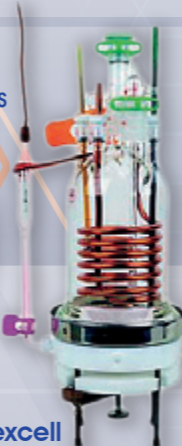
Set-Up for Critical Pitting Temperature Measurements
