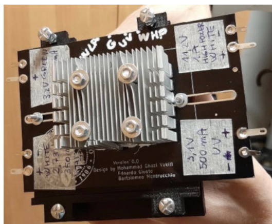
Fig. 3.4 PCB with light source selector and a heat sink
