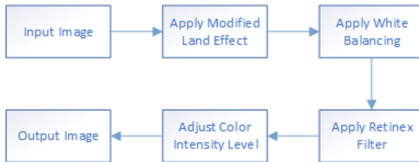
Fig. 2.5 Block diagram of the proposed system
