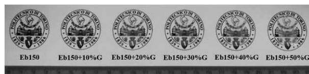
Figure 4: Pictures of UV-LED cured films prepared with different loadings of phosphate glass particles.
