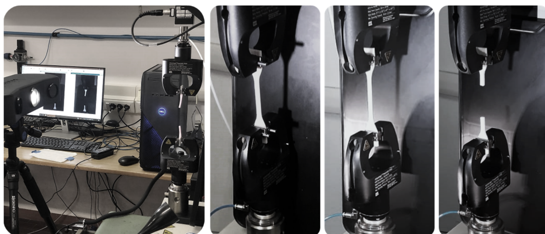
Figure 4. Experimental mechanical testing setup. The deformation of the dog-bone specimen in the initial elastic stage until failure is shown.
