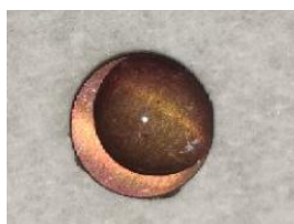
Figure 4.4 Ti64(HF-H 2 O 2 ) with the protein solution drop for KPFM measurement
