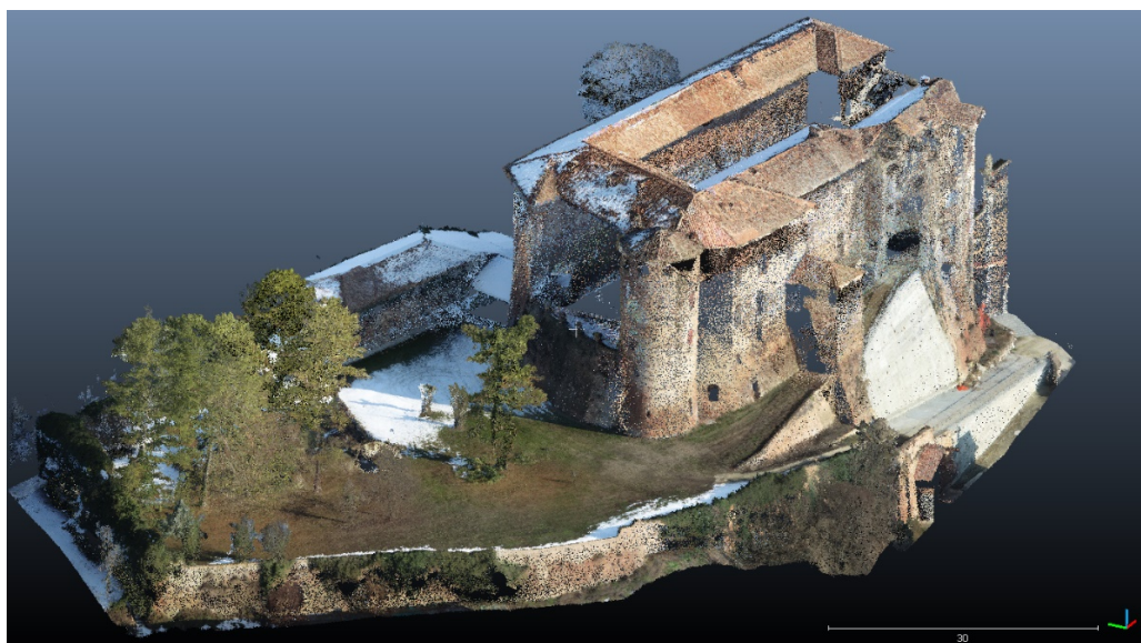
Figure 5. Zenmuse L1 point clouds data related to the castle and the near surroundings within the perimeter walls.
