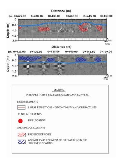
Figure 1. An example of a GPR profile with defect patterns interpretation [14]
