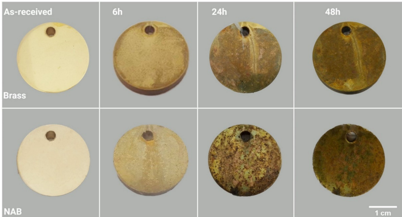
Figure 5. Uncoated samples exposed to the salt spray harsh environment. Both materials start to corrode after 6 h.
