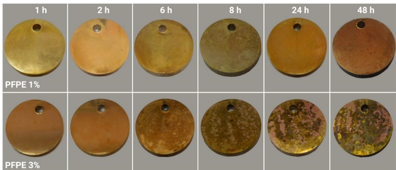
Figure 8. Coated brass samples with two different coatings. PFPE 1% was more effective in preventing corrosion damages.
