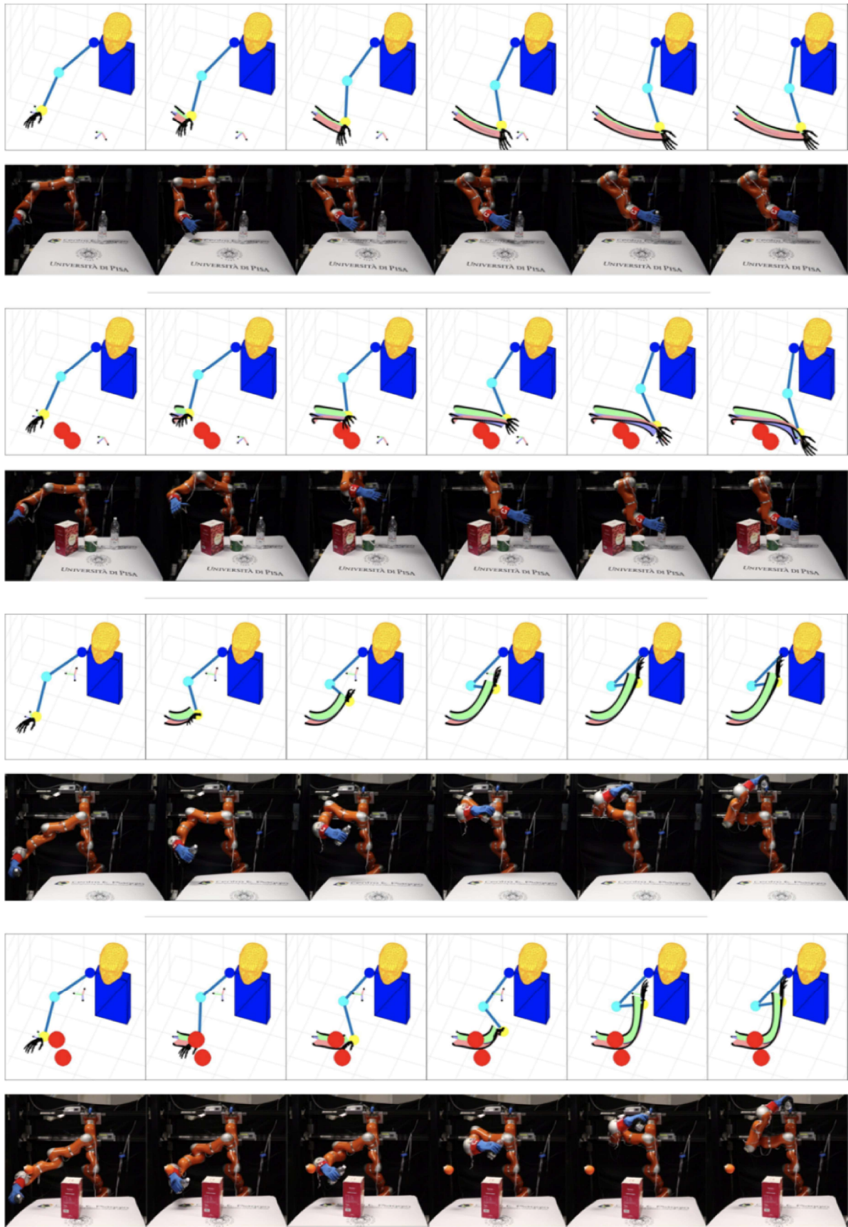
Fig. 5. From top to bottom, snapshots of human reference and real robot execution of T.1 free motion, T.1 with two obstacles; T.4 free motion; T.4 with two obstacles. First controller param: K_x = 100 ; K_y = 100 ; K_z = 100 ; K_{rx} = 1.5 ; K_{ry} = 1.5 ; K_{rz} = 1.5 ; D_x = 2.0 ; D_y = 2.0 ; D_z = 2.0 ; D_{rx} = 1.0 ; D_{ry} = 1.0 ; D_{rz} = 1.0 . Second controller param: K_x = 5.0 ; K_y = 5.0 ; K_z = 5.0 ; K_{rx} = 0 ; K_{ry} = 0 ; K_{rz} = 0 ; D_x = 0 ; D_y = 0 ; D_z = 0 ; D_{rx} = 0 ; D_{ry} = 0 ; D_{rz} = 0 .
