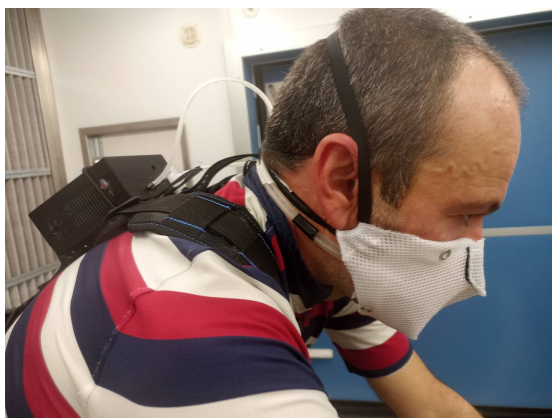
Fig. 5. Sherpa CFC worn by an athlete during submaximal test. Sampling lines for the measurement of pressure and CO 2 concentration are routed inside the mask and their openings are in front of the mouth.
