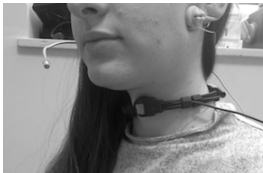
Fig. 2.1 Contact microphone and microphone in air positioning
