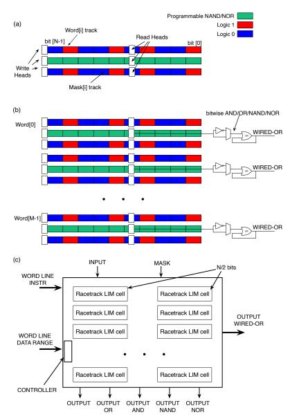
**Figure 11.** (a) Schematic representation of the racetrack memory word with computing capabilities. The central racetrack program the logic function implemented; (b) Racetrack computing array with external logic to complement the computing capabilities able to perform the wired-or. (c) Schematic representation of the logic-in-memory architecture exploiting the racetrack memory.
