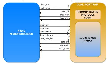
Figure 7. RISC-V-logic-in-memory interface implementation.
