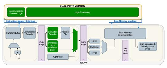
Figure 2. RI5CY core with modified blocks highlighted in green.
