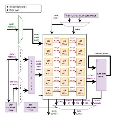
Figure 3. Dual port logic-in-memory high level architecture.
