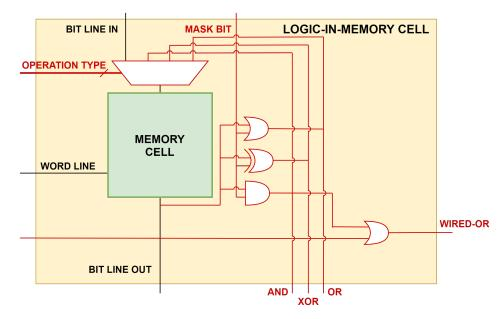
Figure 4. Logic-in-memory bit-cell.
