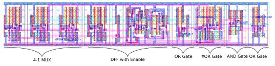
Figure 12. Layout view of the LiM Cell.
