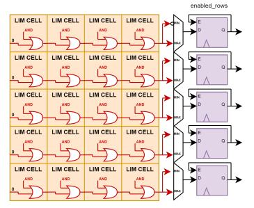
Figure 5. Around-array logic for max-min computation.
