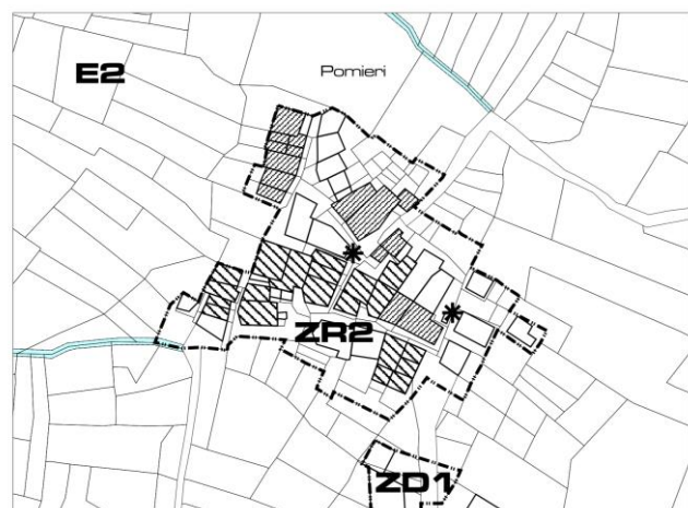
Figure 8. Recovery and developments area of Pomieri (scale 1:1000), ZR2 express Recovery areas and ZD1, development zone, * are fountains or ovens. Buildings on the north need philological restoration, and buildings in the south of the hamlet need conservative renovation activities.
