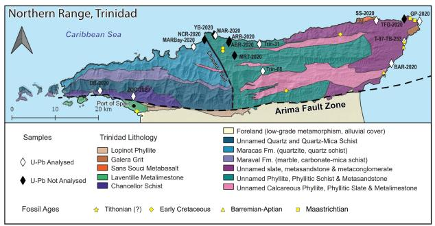
Figure 4. Lithology map of the Northern Range, Trinidad (modified from Gennaro et al. in review). Diamonds show locations of 16 samples from the Northern Range that were collected; 10 of the 16 samples were analyzed for U-Pb age determination. Yellow symbols show 11 fossil locations and their approximate ages from previous research. Black lines represent faults that have been identified throughout the Northern Range.
