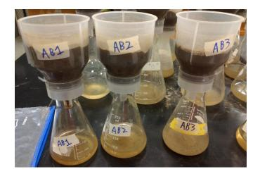
Figure 5: The above figure shows the apparatus for the rain simulation procedure.
