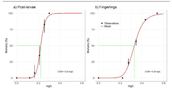
Fig. 1 Concentration-mortality modeled curves (red line) and observation (black points) for both acute toxicity tests. The values of  $LC_{so}$  are also indicated (green line).
