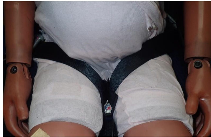
Figure 3. Test setup of the MAMA-2B dummy with the lap belt passed across both thighs and anchored between them using an extra restraint device.
