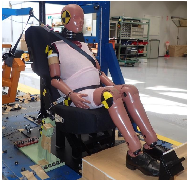
Figure 1. Version 2B of the Maternal Anthropometric Measurement Apparatus (MAMA-2B), restrained in the test setup using a correctly positioned conventional seatbelt.
