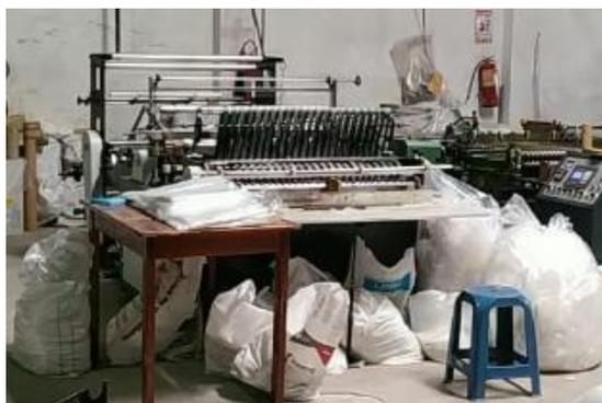
**Figura 20-3.** Máquina selladora LSR multifunction computer heat
