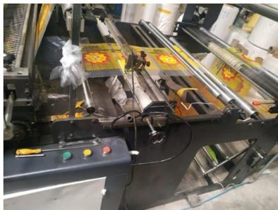
**Figura 15-3.** Máquina selladora LSR multifunction computer heat cutting BAG-MAKING
