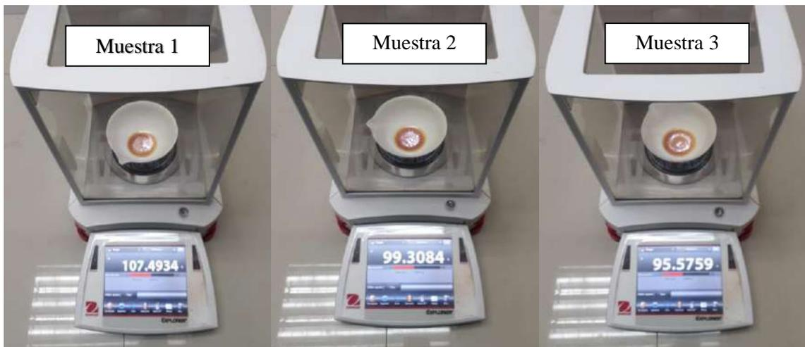
$$ST \text{ muestra}_1 = \frac{107.4934g - 107.4169g}{3 \text{ ml}} \times 100 = 2.55 \%$$
