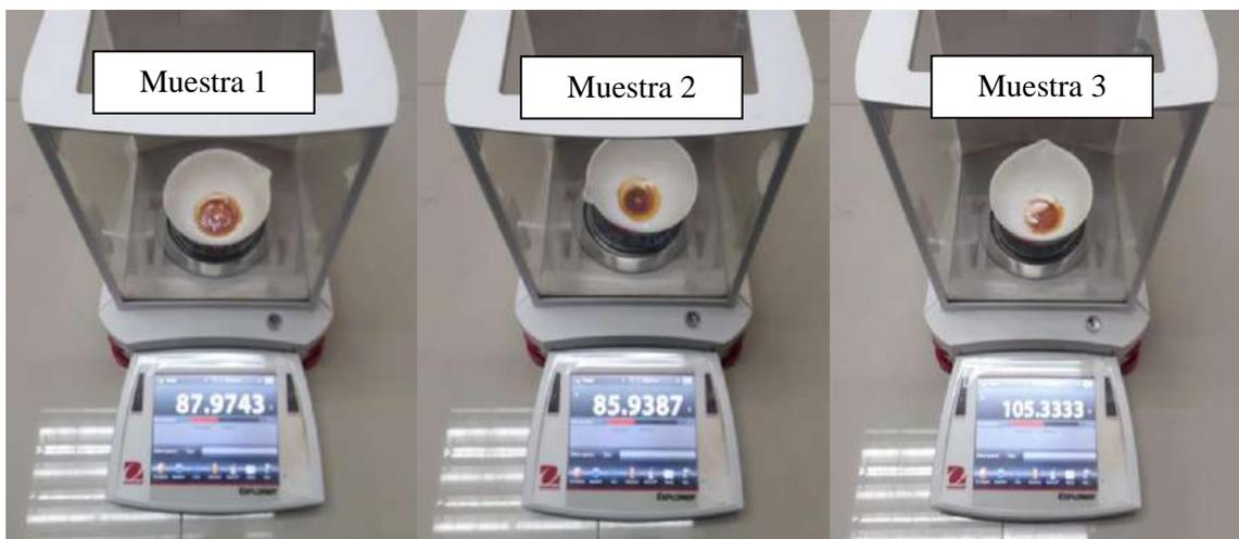
$$ST \text{ muestra}_1 = \frac{87.9743g - 87.8996g}{3 \text{ ml}} \times 100 = 2.49 \%$$
