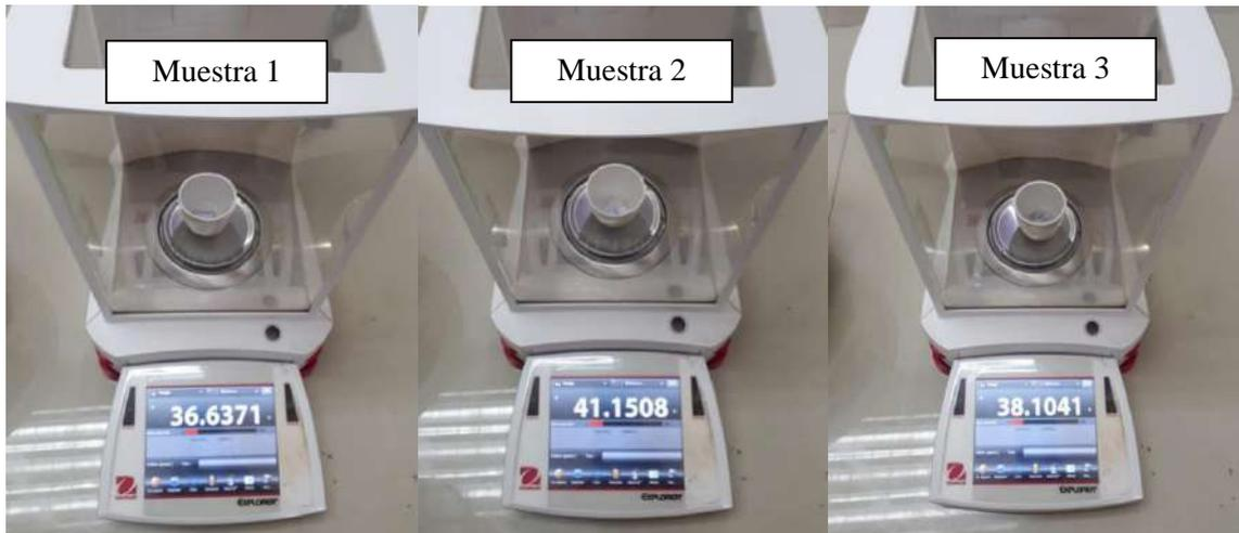
$$\%Ca \text{ muestra}_1 = \frac{36.6371 \text{ g} - 36.6103 \text{ g}}{38.4421 \text{ g} - 36.4410 \text{ g}} \times 100 = 1.33 \%$$
