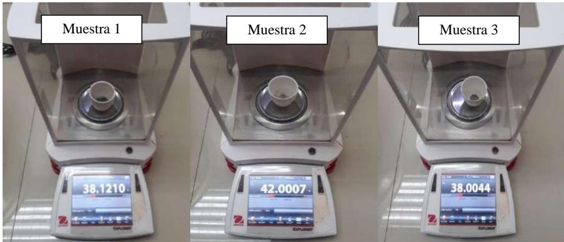
$$\%B \text{ muestra}_1 = \frac{38.1210 \text{ g} - 38.1043 \text{ g}}{40.1243 \text{ g} - 38.1043 \text{ g}} \times 100 = 0.82 \%$$
