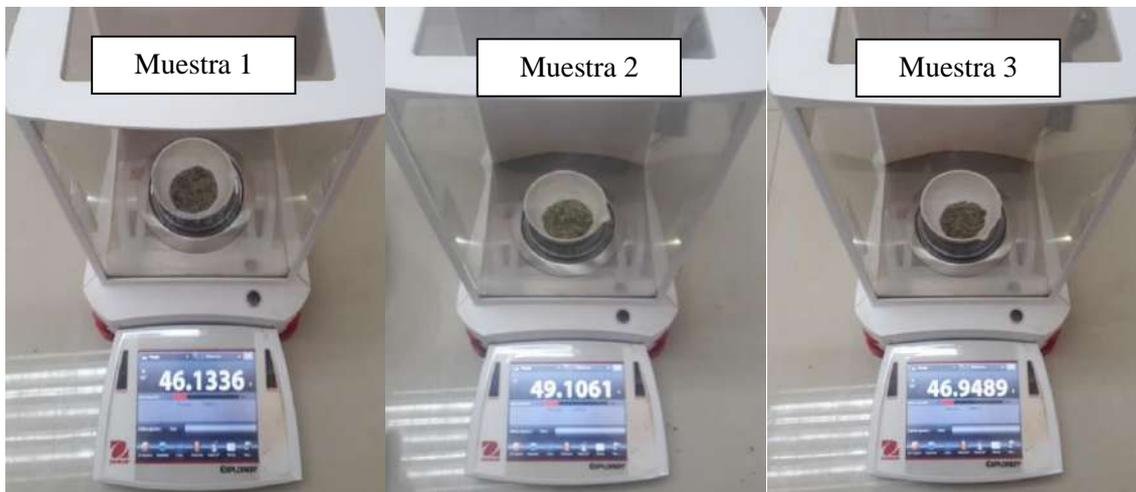
$$\%H \text{ muestra}_1 = \frac{46.2880 \text{ g} - 46.1336 \text{ g}}{46.2880 \text{ g} - 44.2872 \text{ g}} \times 100 = 7.72\%$$
