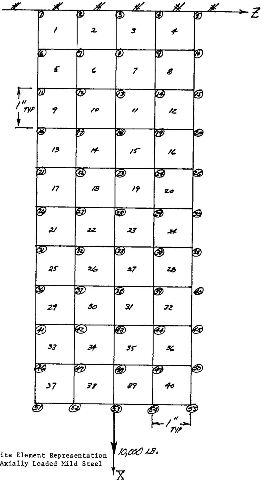
Figure 4 : Finite Element Representation of Axially Loaded Mild Steel Rod
