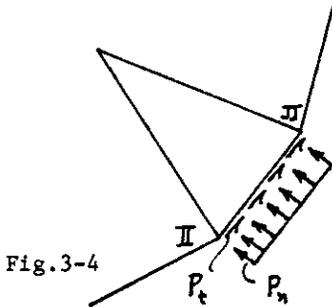
The boundary element must be on the left as one progresses from II to JJ. Surface tensile force is input as a negative pressure. Positive shear pressure is in the direction from II to JJ.
