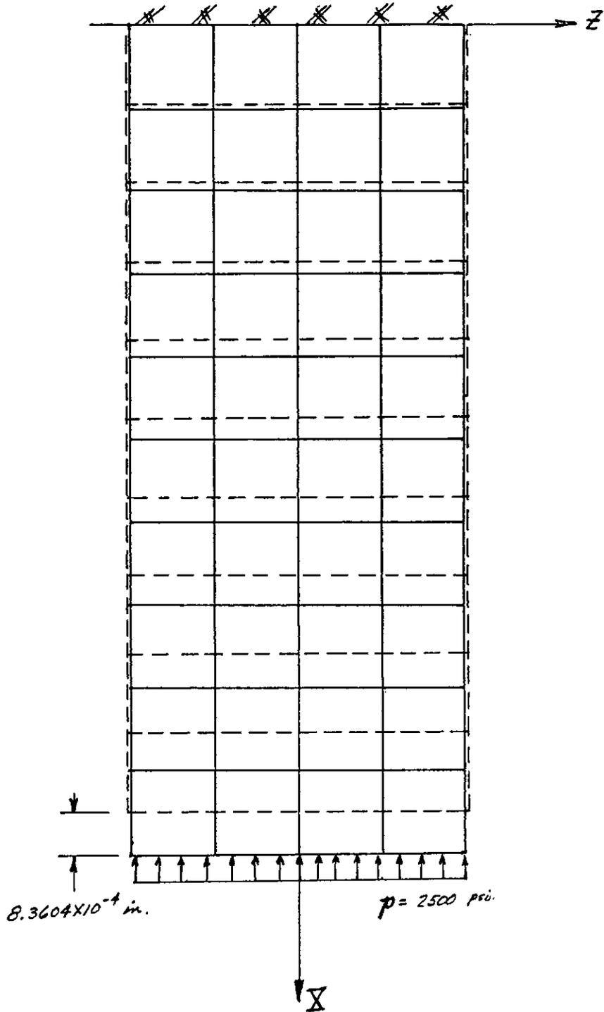
Figure 7 : UNIFORMLY LOADED ROD WITH DISPLACEMENT
