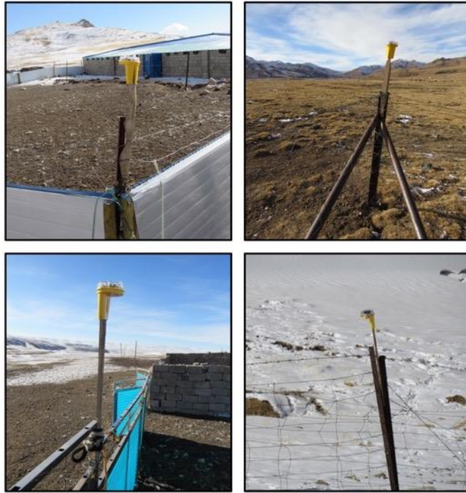
Figure 37. Examples of congruency in Foxlight installation among herders in the experimental group. Foxlights were installed in either corners or entry points of night time pastures at heights ranging from 1.7 to 2.5m from the ground to remain visible to wild predators.
