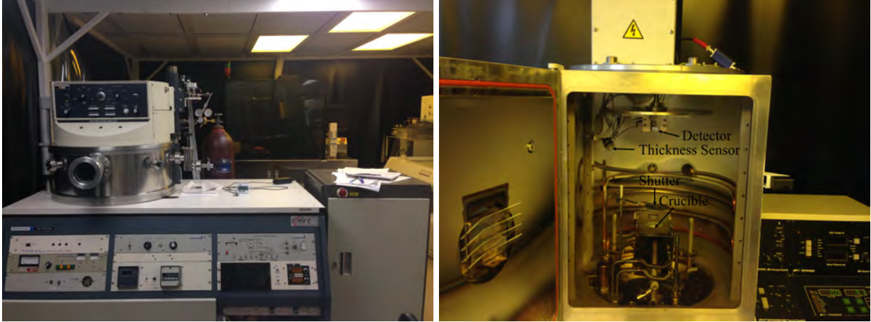
FIGURE 3.4: Shown are the equipments used to carry out the contact formation on the high-purity germanium crystal. Left: Perkin Elmer (2400 model) Sputtering machine at USD used for the a-Ge and Al deposition; Right: Electron-Beam machine at USD used for the Al deposition on top of a-Ge contacts.
