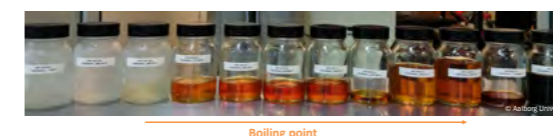
Fig. 2: Distillation products of upgraded HTL biocrude.
