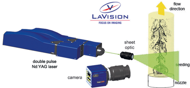
Figure 6.6-4: System components of Particle Image Velocimetry (Source: Lavisoin GmbH 2018)
