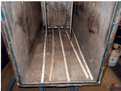
Figure 8.7-6: Dry digester pilot vessel with slotted PVC piping on the floor and the floor grating in the background. The rods that pull down on the compression grating system are also visible (Source: InnoTech)
