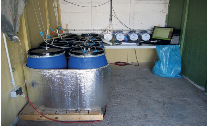
Figure 5.4-2: Manure storage test stand (Source: DBFZ 2018)
