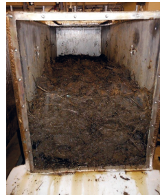
Figure 8.7-16: Digester 1 and Digester 2, open at the end of the trial with post digestion contents visible (Source: InnoTech)
