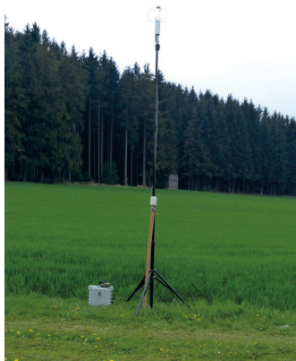
Figure 5.6-1a: Weather station (Source: DBFZ)
