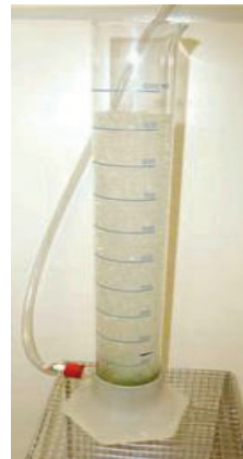
Figure 6.3-2: Foam generator with model foam (Source: UFZ)
