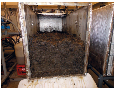
Figure 8.7-16: Digester 1 and Digester 2, open at the end of the trial with post digestion contents visible (Source: InnoTech)
