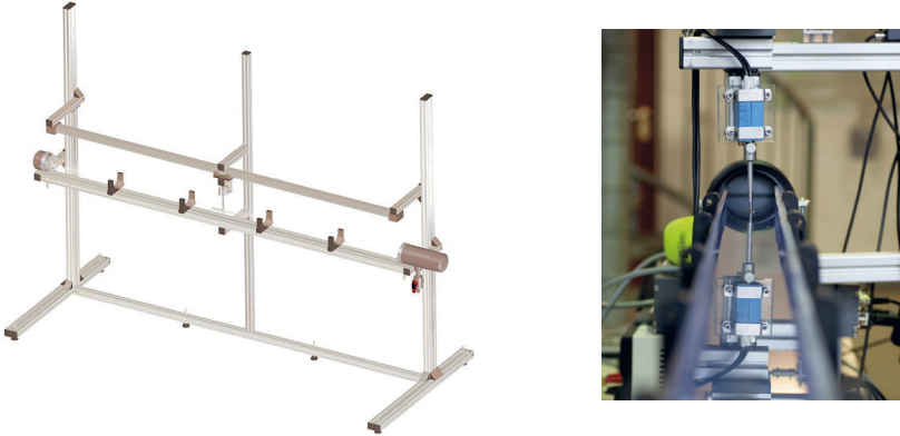
Figure 6.6-6: Towing-channel for the calibration and determination of the constants of a film sensor
