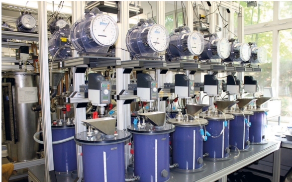
Figure 7.4-2: Laboratory for continuous fermentation tests at the DBFZ
