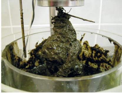
Figure 6.5-6: Wrapping of the vane shaft with long fibre substrate components (Source: BREHMER)
