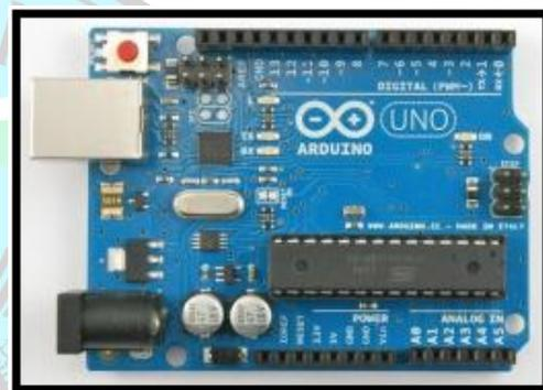
**Gambar 3.** Papan Arduino Uno
