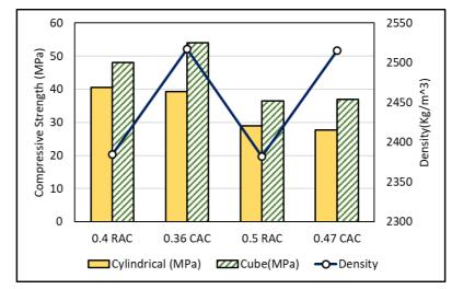
Fig-2: 28-day cylindrical and cube strength and Hardened density of the mix
