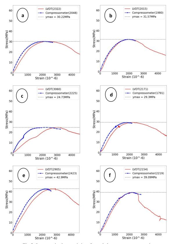
Fig-5: Stress-strain characteristics of recycled aggregate concrete mix
