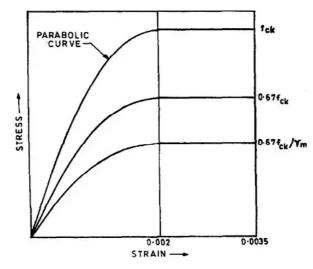
Fig-10: Standard Stress-Strain characteristics of concrete assumed in IS 456
