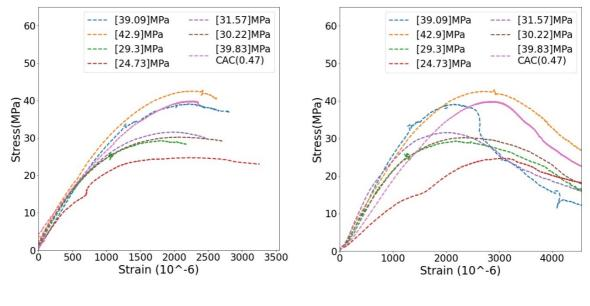
strain curve but fails with the initiation of initial crack in the specimen. Therefore a compressometer is not capable of capturing the post peak behaviour.
