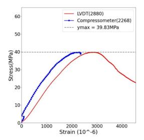
**Fig-6**: Stress-strain characteristics of natural aggregate concrete mix (w/c = 0.47) [21]
