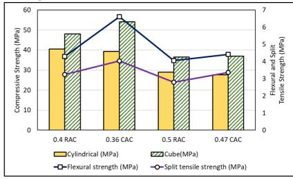
Fig-4: Flexural and Split Tensile strength
