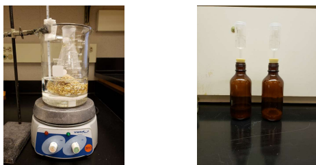
Figure 1. The image on the left shows the set up used to prepare the fermentation. The image on the right shows two bottles with bubblers that held the fermenting solution and the headspace gas
