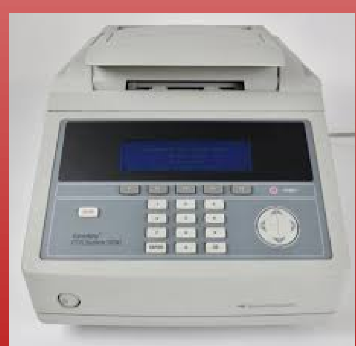
Figure 1. PCR Thermocycler was used to dry sugars out of aqueous solution, and then to heat the derivatized mixture.
