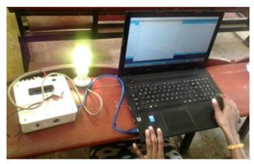
Figure 8: Using GSM-HAS to control the appliance
