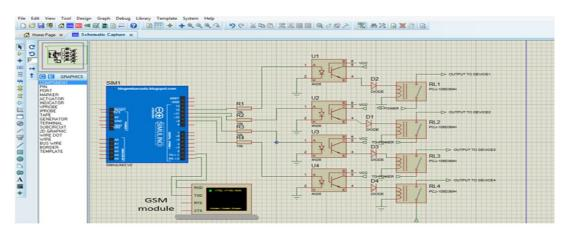
Figure 5: Image of Proteus software for circuit development
