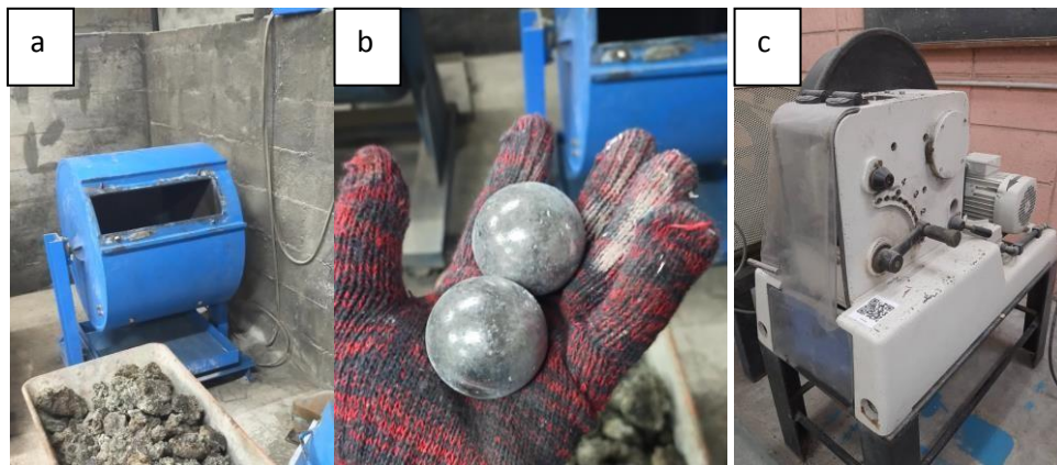
Figure 5. (a) Los Angeles Abrasion Testing Machine, (b) ball bearings, (c) stone crusher machine
