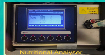
Nutritional Analyser Milk is checked for nutritional content
