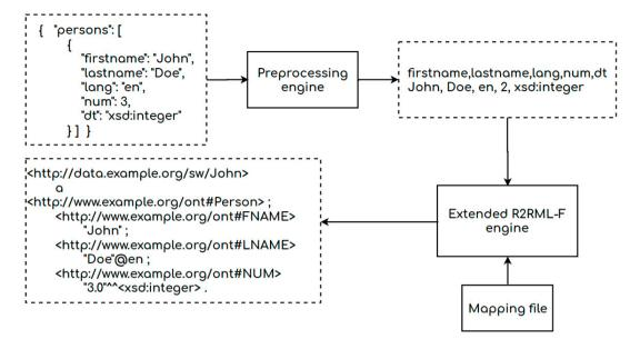
Fig. 2. Illustrative example of extended R2RML-F
