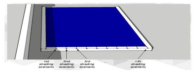
Figure 5. Influence of shading effect on PV modules (Topić, 2017)
