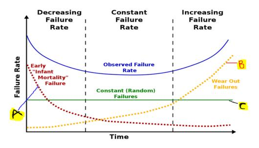
Figure 2. Multiple failure modes overlap of solar PV modules (Allen and David, 2015)
