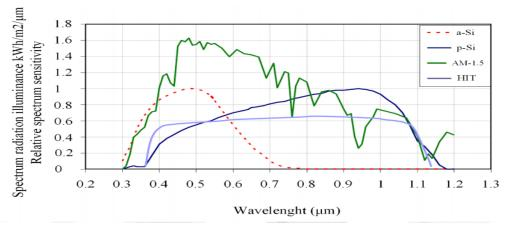
Figure 4. Spectrum response of different PV technologies (Sirisamphanwong, 2013).
