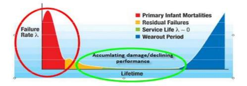
Figure 1. "Bathtub" curve for PV Durability and Reliability (Allen and David, 2015).
