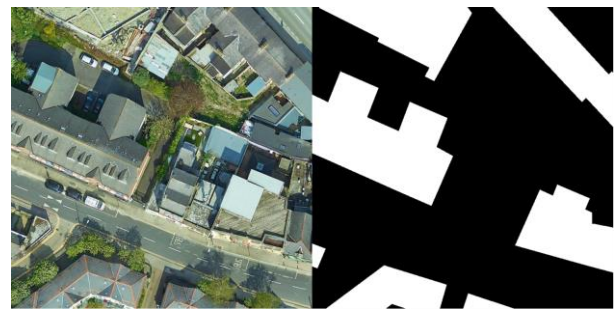
Figure 8: A data sample from the OSM-GAN training dataset. The left side is the input Google satellite image – the right side is a binary image of the current OSM building footprint (feature-map) of the area.
