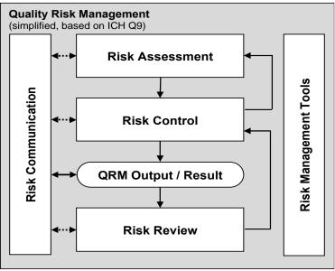
Figure 1 - The QRM Process Model (simplified) [1]
