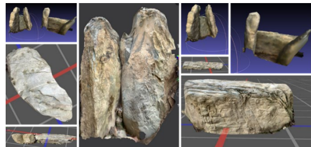
Figure 7. Textured meshes of a range of exposed structural stones from Dowth Hall, created using the iPad Pro in conjunction with the 3D Scanner App and MeshLab.
