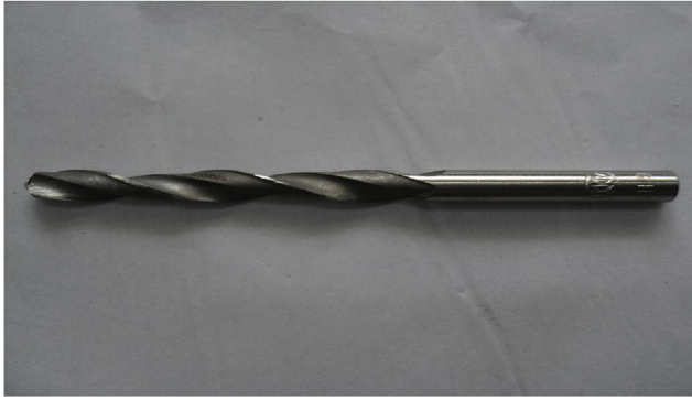
Fig. 3 – Cryogenically treated 6 mm drill bit.
