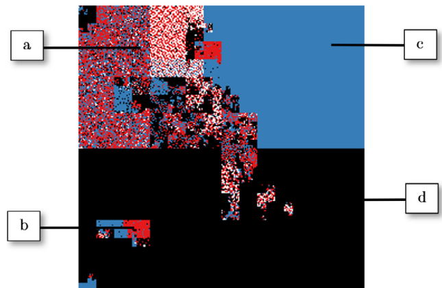
Fig. 3. SFC image mapped from a sample of the Chir worm. a denotes a mixture of data types; b is a region of high value bytes (127–255 range); c is a region of ASCII printable characters; d is a region of null bytes (binary zeros).
