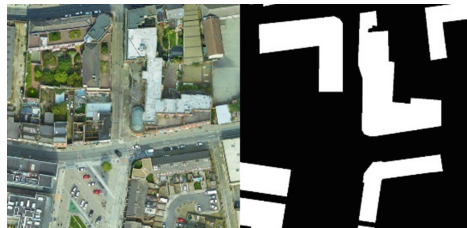
Fig. 2. One sample of the OSM-GAN training dataset. The left side illustrates the satellite image component, and the right side shows the corresponding feature-map .
