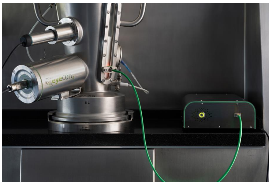
Figure 2: The PAT product bowl with integrated PAT & wiper
