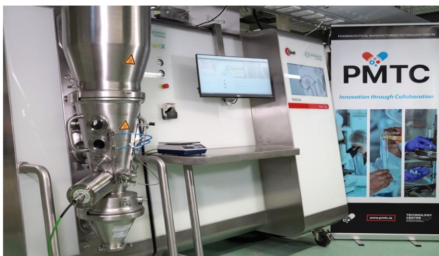
Figure 1: SmartX-equipped fluid bed system at the University of Limerick
