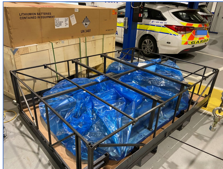
Figure 15: Hyundai EV battery pack ready for shipment. The steel create packaging is an ADR / IMDG requirement, which warrants a high transport cost. Note the “UN3481” ADR designation warning on the box, which will cover the crate. (MMcGuinness, 2021).
