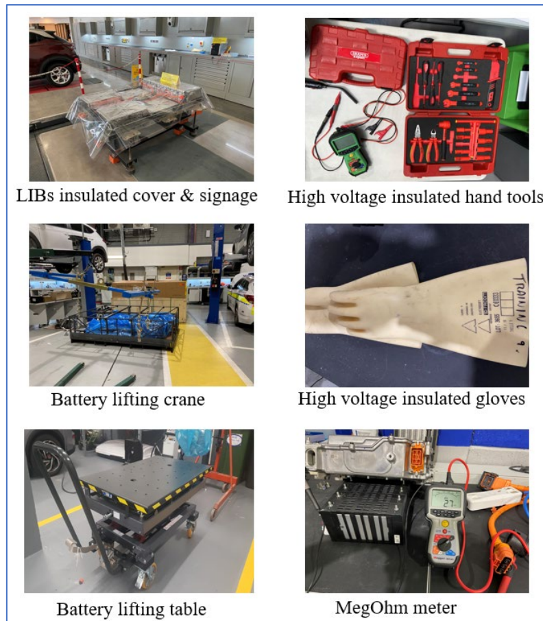
Figure 18: Examples of special tooling and PPE required when working on, or removing EV batteries. The various items are of a considerable cost, which may entice actors to cut corners. The items are from different manufacturers, viewed by the author during site visits (MMcGuinness, 2021)
