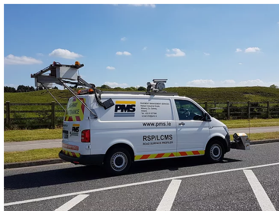
Figure 1: Pavement assessment van with LCMS mounted on the backside.
