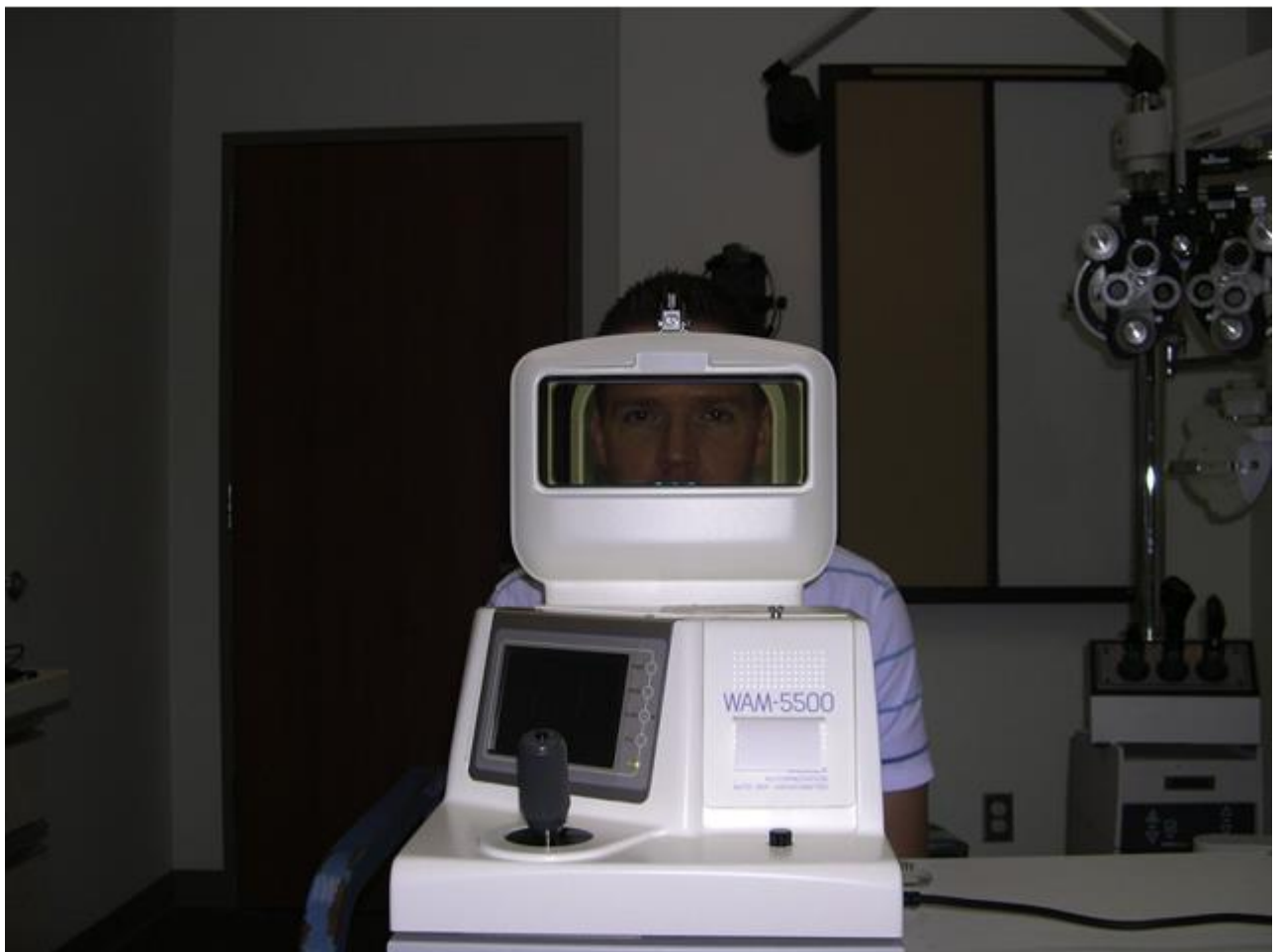
Figure 3.2: An example of an open-field autorefractor, the device recommended by the International Myopia Institute (IMI) to determine refractive error in epidemiological and interventional studies of myopia. 169 Reproduced from Bradley et al. 173
