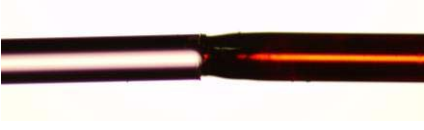
Fig. 4. Image of a chalcogenide multimode fiber with a length of circa 24.75 mm spliced with a silica singlemode fiber.
