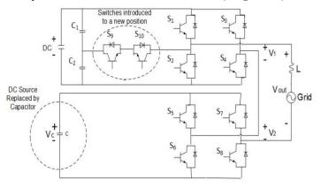
Fig. 1. Proposed Grid-tied Multi-level Topology
