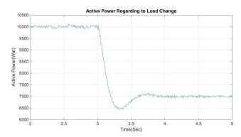
Fig. 4. Active Power to the Grid (Reference Changes from 10kW to 7kW)
