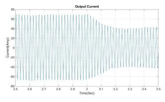
Fig. 7. Inverter Output Current (Reference Changes from 10kW to 7kW)
