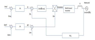
Fig. 3. Control structure for a single phase grid connected MMC
