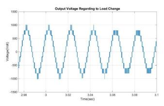
Fig. 6. Inverter Output Voltage with load change at t=3s
