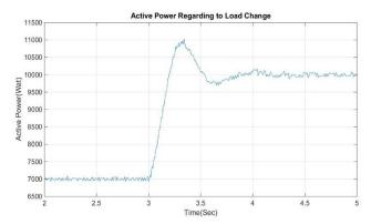
Fig. 9. Active Power to the Grid (Reference Changes from 7kW to 10kW)
