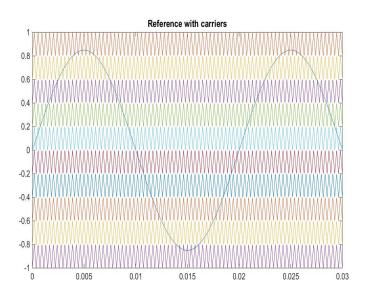
Fig. 2. Reference signal with multi-carrier level shifted PWM
