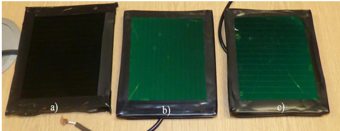
Fig. 1. CdTe mini modules (196 cm 2 ). (a) A clear module, (b) encapsulated with dye-LDS layer and (c) with dye-pLDS composite layer.
