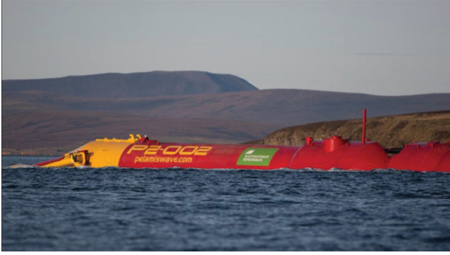
Fig. 1. Photo of the Pelamis wave power device [6]. The device is typically 1600 m from the shoreline.
