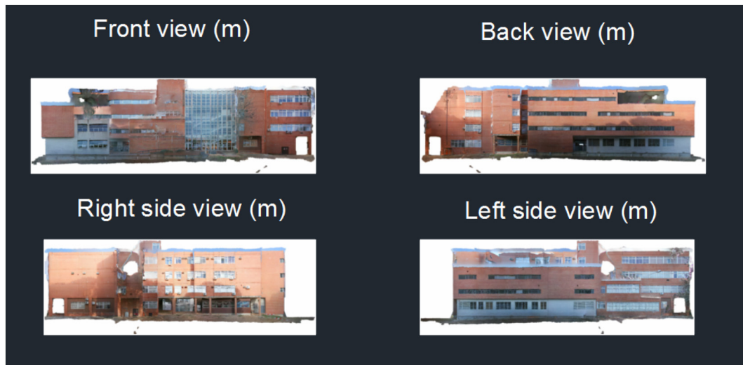
Fig. 3. 2D elevations of the building. Photogrammetry.
