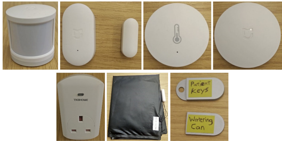
Fig. 1 SCAMPI sensors. Top row (from left to right): motion sensor, door sensor, ambient sensor, button sensor. Bottom row (from left to right): power sensor, pressure sensor, beacon sensors
