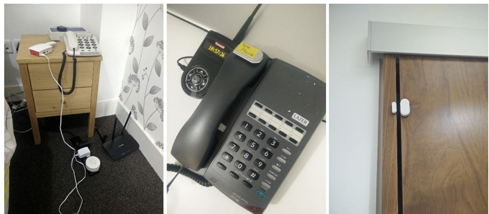
Fig. 4 Deployment of some of the SCAMPI devices in the TECS lab. Left—hub devices. Middle—beacon attached to a telephone. Right—door sensor attached to the bathroom door
