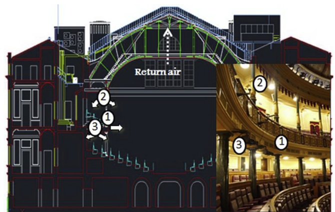
Fig. 2. Position of the supply air outlets and return.
